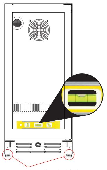
Rotate to raise or lower the LEVELING LEGS located at each of the four corners until all four legs are seated firmly on the floor and the interior floor of the unit is level both front to back and side to side.
