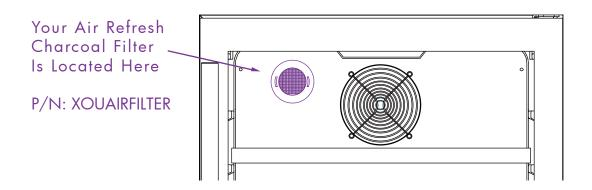
Rotate the filter 1/4 turn to unlock
