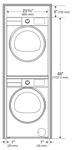
NOTE: Only one electrical outlet is needed since the washer can plug into the dryer. The use of two electrical outlets may be used as an alternative.
