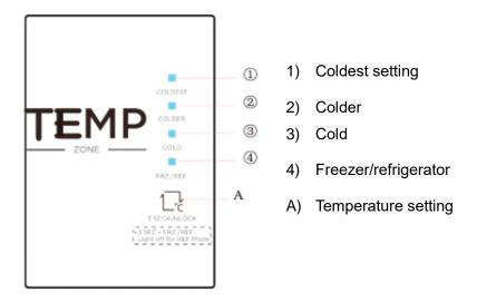
Once powered on, the display screen will fully display for three seconds, and then the normal operation functions will display.
