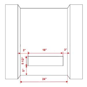
Required minimum air gap clearances: 1/4" sides
