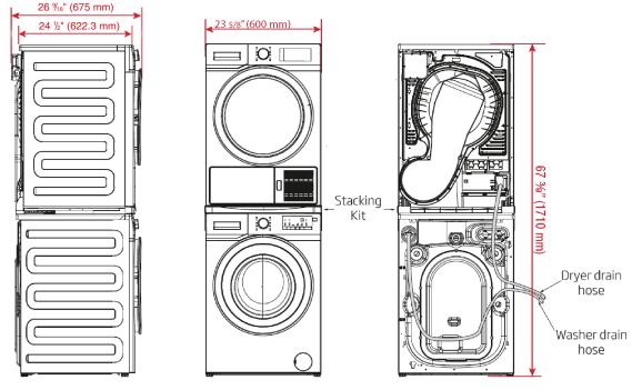
Stacked installation minimum air gap clearances: 6 ¼" top, ½" sides, ½" back, front ½"
