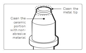
Do not cook while you clean the cooktop. Ensure the white ceramic electrodes are clean and dry. Clean the metal with a soft cloth. Do not clean the igniters with water.
