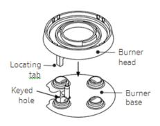
1. Place the burner heads as shown. The locater tab on the head goes in the keyed hole as shown.
