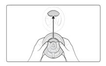
1. Orient the burner head so the electrode opening aligns with the electrode itself.
