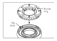
2. Put the burner rings on the heads as shown. Match the tabs on the bottom of the ring to the slots on the head. Wiggle each ring to ensure it is properly seated.
