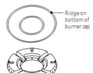
3. Put the burner caps on the burner rings. The ridge around the bottom edge of the cap fits around the top of the ring.
