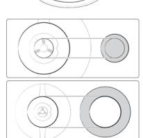
3. Size the burner caps to the burners, then re-install them on the heads.
