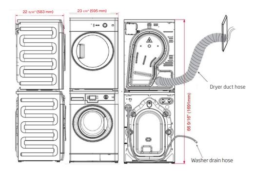
Required Minimum Air Gap Clearance: 1 " (25.4 mm) Top (when placed side-by-side or stacked)  $J_2$ " (13 mm) Sides 4" (102 mm) Back with 90° elbow
