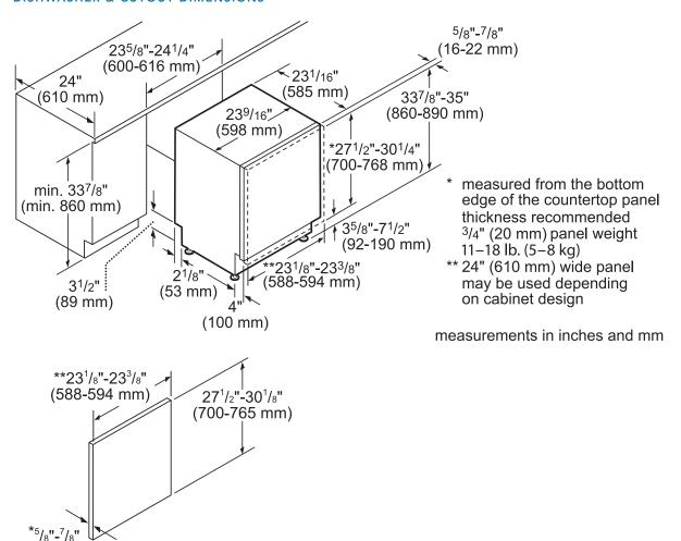
\* thickness recommended <sup>3</sup>/4" (20 mm), panel weight 11–18 lb. (5–8 kg)
