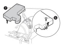
3 Remove the cover and pull out the tube <sup>(3)</sup>. Disconnect all wire harnesses <sup>(2)</sup>. Unscrew the ground wire <sup>(1)</sup>.
