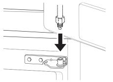
2 Fit the hinge **1** over the hinge lever latch **2** and slot it into place. Rotate the lever **3** counterclockwise to secure the hinge.
