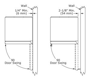
Units have a zero clearance for the door to open  $90^{\circ}$ , when installed adjacent to cabinets.
