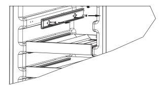
5. Place the spacer in between the liner and slide.
