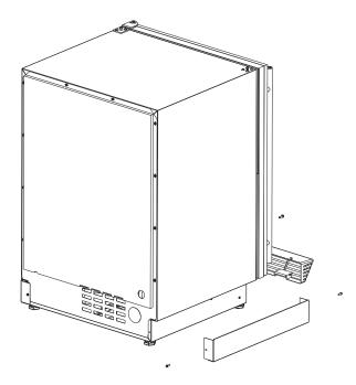
3. Align front hole with hole in shell accessory, hole in base, and hole in grille. Tighten screw.
