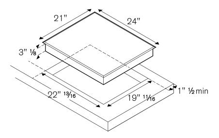
Bertazzoni recommends to operate the appliance after it has been installed in a cabinet. The kitchen cabinets shall be made of materials capable of withstanding temperatures at least 117°F (65°C) above room temperature in order to avoid possible damage to the cabinets during appliance usage. For further installation instructions refer to the installation manual.
