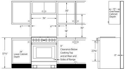
\* Side clearance above cooking surface to any objects, i.e., wall.
