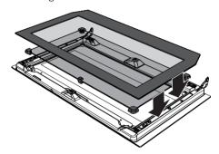
6. To put back the internal glass pane, slide the upper part into the door strip and insert the two rear pins into their seats by pressing lightly.
