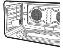
Spray a water and washing up liquid solution inside the oven using a spray nozzle. Direct the spray towards the side walls, upwards, downwards and towards the deflector.
