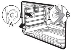
When you have finished cleaning the oven, repeat the procedures indicated above in reverse to replace the guide frames
