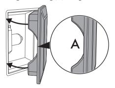
7. Press the cover firmly so that it adheres tightly to the light bulb holder.
