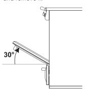
3. To reassemble the door, put the hinges in the relevant slots in the oven, making sure that the grooved sections A are resting completely in the slots. Lower the door and once it is in place remove the pins from the holes in the hinges.
