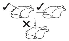
In order for the probe to measure the core temperature of the food precisely, its tip must not be in contact with bones or fat.
