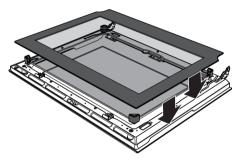
6. Replace the inner glass panel. Make sure you center and insert the four pins into their grooves in the door, using a little pressure.
