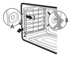
• When you have finished cleaning the oven, repeat the procedures indicated above in reverse to replace the guide frames.
