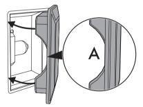
7. Press the cover firmly so that it adheres tightly to the light bulb holder.
