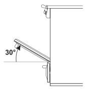
To reassemble the door, put the hinges in the relevant slots in the oven, making sure that the grooved sections A are resting completely in the slots. Lower the door and once it is in place remove the pins from the holes in the hinges.
