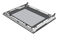
5. Reinsert the glass panels in the reverse order of removal.
