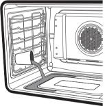
Spray a water and washing up liquid solution inside the oven using a spray nozzle. Direct the spray towards the side walls, upwards, downwards and towards the deflector.
