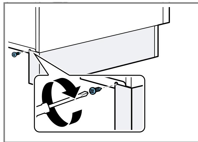
3. Remove and retain screw in right/left side frame.
