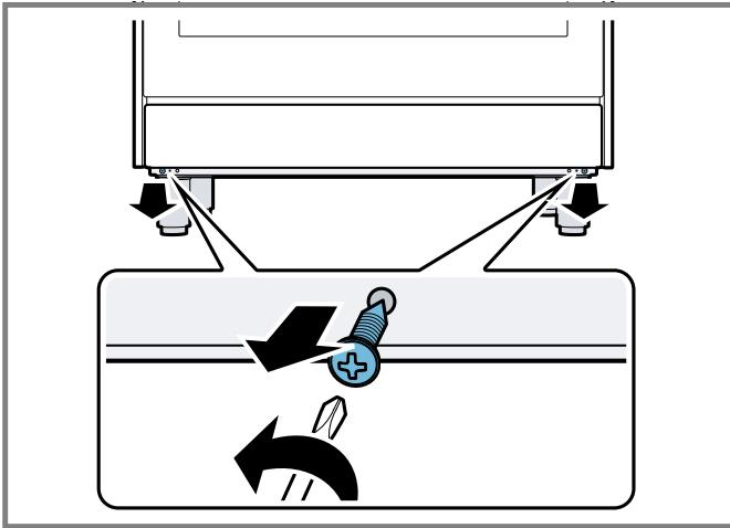
2. Fix the front toe kick plate using the screws removed in step 1.
