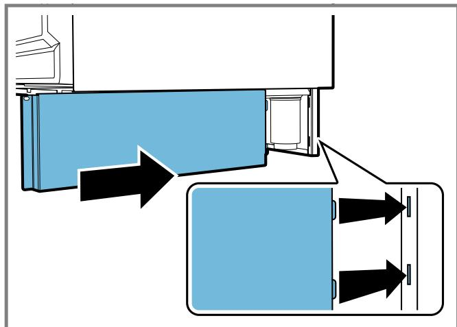
5. Fix the right/left toe kick plate using the screw removed in step 3.
