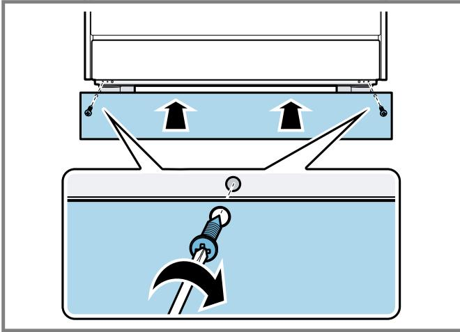
3. Remove screw shown in diagram below from each side in preparation to install left and right toe kick support brackets.
