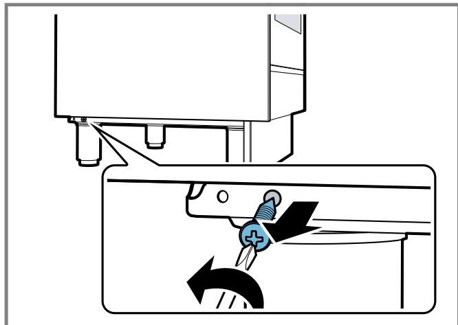
4. Take the right/ left side toe kick plate and rotate it in order to insert the tabs into the slots of the front toe kick plate.
