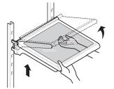
**2** Pinch the sides to open the water filter cover.
