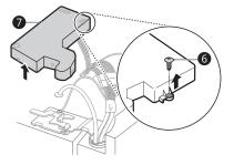
3 Remove the cover and pull out the tube 3. Disconnect all wire harnesses 9. Unscrew the ground wire 1.
