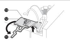
**5** Lift the door from the middle hinge pin and remove the door.
