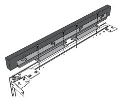
Align the front of the panel with the appliance door using the slots on the bracket.
