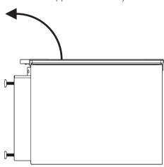
8. If it is not already mounted, fasten the bracket **C** to the top of the appliance using the screws supplied as shown in the figure below.
