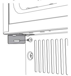
12. Fasten the appliance also to the side walls of the cabinet with the screws provided using the upper fixing plates.
