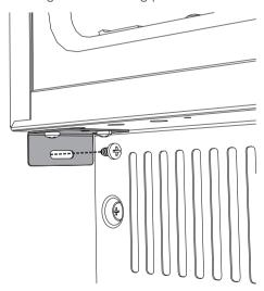
12. Fasten the appliance under the top of the cabinet with the screws provided using the upper bracket.
