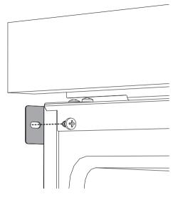
13. The upper fixing plate near the door hinge must be fastened through the gap between the door and the appliance.
