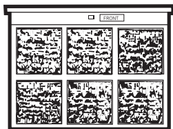
Dirty filter— Needs cleaning
