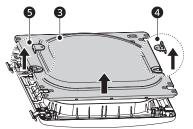
Remove the 4 screws is securing the hinges to the door frame. Remove the two plastic cover caps in the ninges is and cover caps in the opposite sides from which they were removed.
