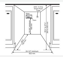
If the drain outlet is higher than 24" (610 mm), the connections will need to be recessed.
