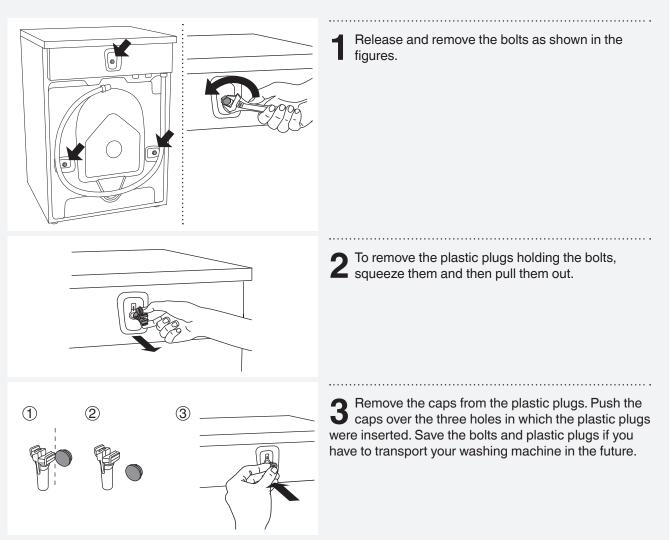
$\dot{\gamma}$  If you wish to transport the washing machine, reinstall the bolts and plastic caps to lock the machine. This will prevent any damage to the machine due to vibrations during transport. If you have lost the transport bolts or plastic caps, replacements can be ordered at your dealer.
