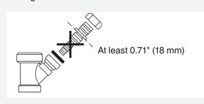
$\overline{\ }^{-}$  If the hose is extended, the internal diameter of the coupling must not be less than  $\frac{1}{2}$ " (12.2 mm).
