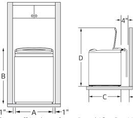
To ensure sufficient clearance for water lines and airflow, allow minimum clearances
